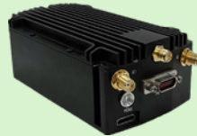
11.7×6.2×3.8cm/349g 11.7×6.2×4.2cm/360g 1Watts×2/2Watts×2 Extended WIFI/HDMI/SDI (Air to G. 20~50/50~100KM)
