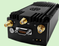
11.7×6.2×4.2cm/380g 2Watts×2/4Watts×2 Extended WIFI/HDMI/SDI (Air to G. 20~100/100~150KM)
